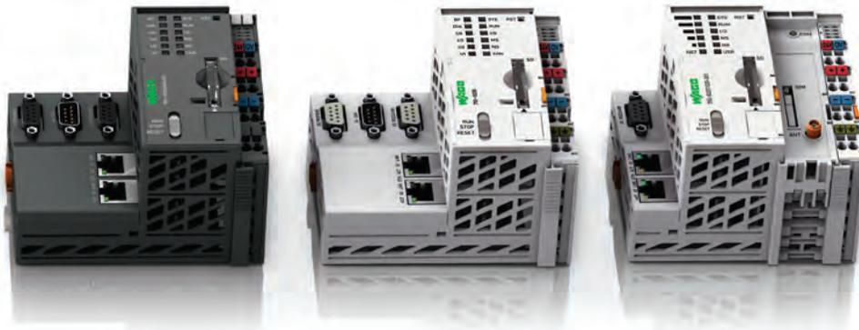
The impressive PFC200 Controller features a high processing speed and a large selection of interfaces. The CANopen, PROFIBUS DP, MODBUS TCP/UDP/RTU and Ethernet/IP protocols provide flexible connection to fieldbus systems and external input/output devices. And multiple variants – including the extreme temperature range (XTR Series) – provide these features for virtually any application.
